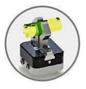
It can also be used as a parallel gripper, centering and positioning element, since the same forces are always generated, regardless of whether centering is carried out inside or outside.
