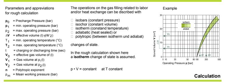
For all accumulator calculations following absolute pressures should be used (**relativ + 1 bar**). The temperatures  $T_1$  and  $T_2$  in ° Kelvin (T + 273).
